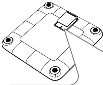
If you would like to change the measurement unit, you can press the button in the battery compartment to cycle through pounds, kilograms or stones.
