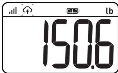
During transmission, the scale display will flash the
