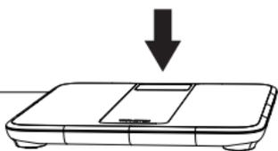
Lay the scale on flat and level ground away from water or other hazards.
