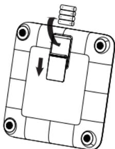
Insert four AA batteries into the back of the scale.
